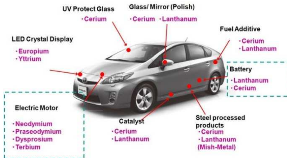
Figure 1. Critical elements used in various components of a modern motor vehicle Source: Universiteit Leiden ( https://www.universiteitleiden.nl/en/research/research-projects/science/cmlrare-earth-supply-chain-and-industrial-ecosystem-a-material-flow-assessment-of-european-union )
